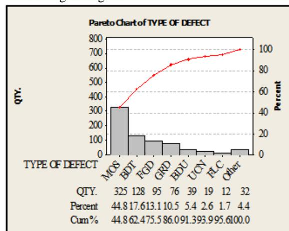
Fig.3 Pareto diagram modes of defects of Taper Shank Drills.
