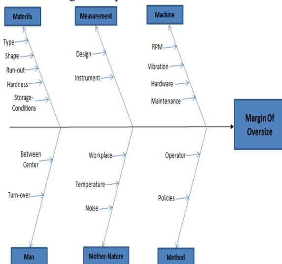
Fig.5 Cause-and-effect diagram
